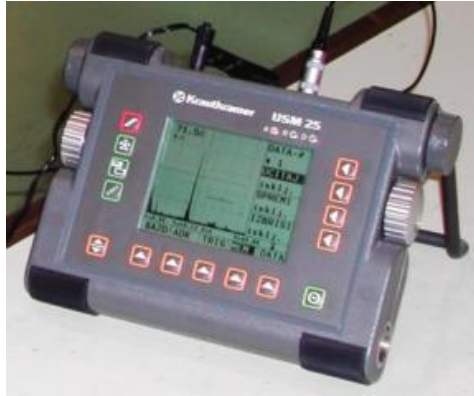
Ultrasound inspection device KRAUTKRAMER USM-25
