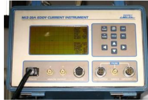
Eddy current inspection device ZETEC MIZ-20A
