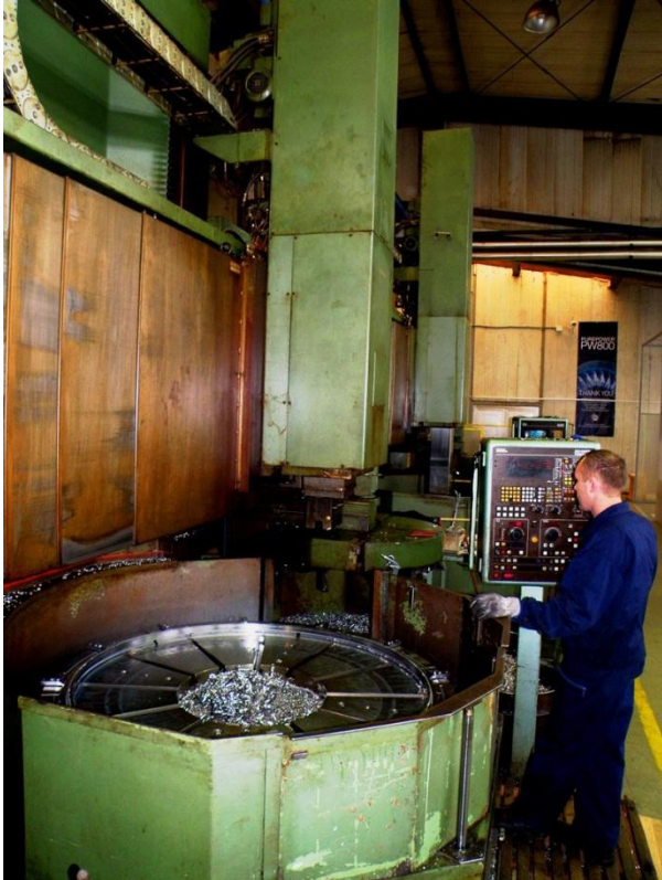
Turning diameters up to 1600 mm
