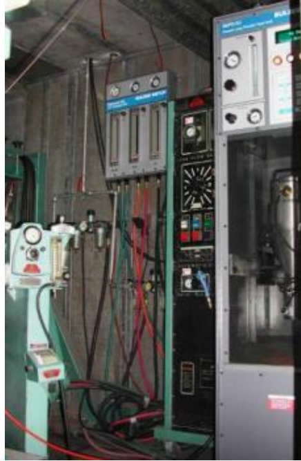
Plasma (by wire or powder feeding) & HVOF coatings by METCO Diamond Jet equipment)
