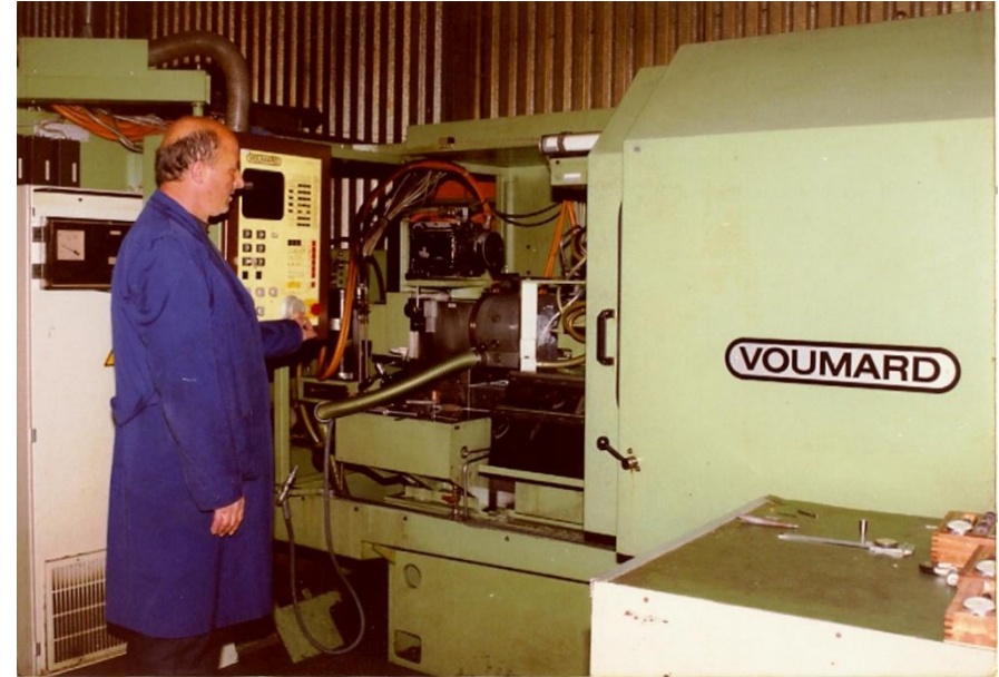
Cylindrical and flat grinding accuracy up to 0.005 mm.
