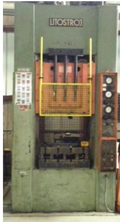
LITOSTROJ hydraulic press–force up to 100 MPa
