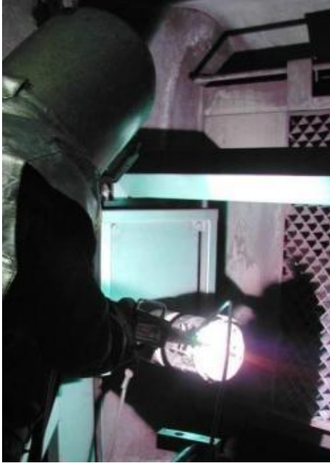
Plasma (by wire or powder feeding) & HVOF coatings by METCO Diamond Jet equipment)
