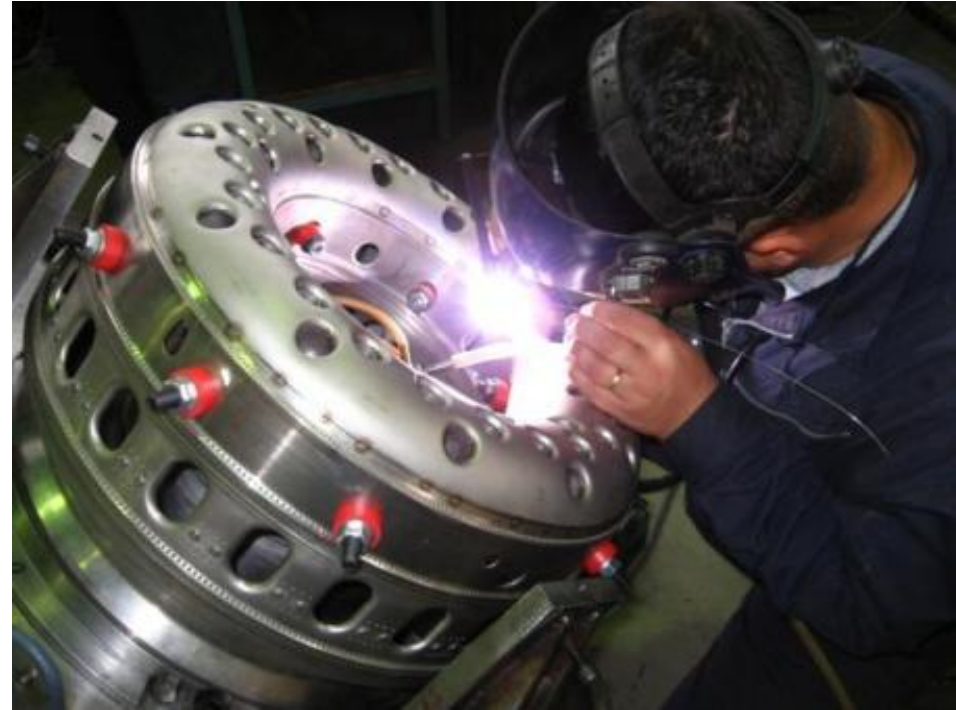
Manual TIG welding of front section combustion chamber of Viper 632-43 turbojet engine
