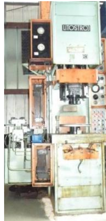
LITOSTROJ hydraulic press – force up to 63 MPa
